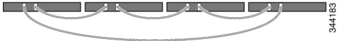
Figure 9: Data Stacking in a Side-by-Side Mounting
